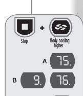
In order to read out the counter of the tubes, the "stop" button and the "body cooling higher" button must be pressed simultaneously for three seconds.
